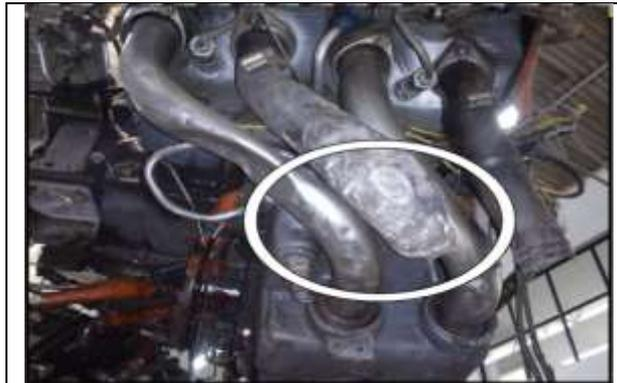
***Induction tube and exhaust tube was sheared off***
