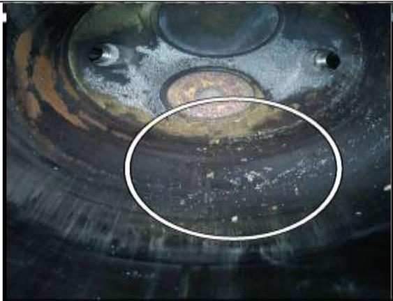
***Dust like material observed inside Combustion chamber***
