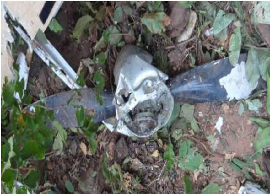
***Sudden impact of propeller shows breaking of shaft under power***
