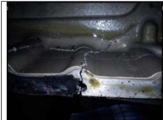
***Top reservoir was cracked which might have caused oil to drain out***
